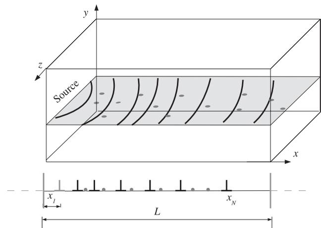
FIG. 1. At the top, we show a three dimensional sketch of a slip plane line containing a pileup of dislocations emitted by a source placed on the left surface and absorbed at the right-hand side of the sample. Our simplified model is shown in the bottom part of the figure: dislocations move on a line of length  $L$  and interact with each other, with image dislocations and with point impurities. The source is modeled as an immobile dislocation with varying Burgers vector placed at  $x_1$ .
