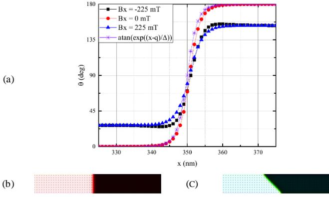
Fig. 1. Characterization of the static DW structure under the application of in-plane fields along the length of the wire. (a) Change in the spherical coordinate  $\theta$  at the center of the wire under different longitudinal fields compared to the conventional Bloch DW profile [3,4], (b) DW structure under  $B_x = 225$  mT, (c) DW structure under  $B_x = -225$  mT.
