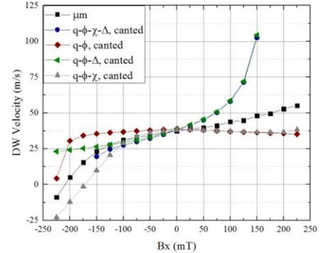
Fig. 2. Variation of DW velocity with in-plane field. Simulations were performed for a current density of  $J = 0.1$  TA/m<sup>2</sup>.
