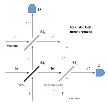
FIG. 2. (Color online) Model scheme of a realistic Bell measurement. The model takes into account the non-unity efficiency of the detectors D performing the homodyne measurement. In the depicted scheme, such inefficiency is simulated by the introduction of two fictitious beam splitters, BS<sub>2</sub> and BS<sub>3</sub>, with equal transmissivity  $\eta$ .
