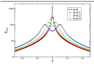
FIG. 3 (color online). Average fidelity susceptibility for various disorder strengths  $\sigma \in \{0, 0.1, 0.2, 0.3\}$ , with fixed system size L = 400. Here  $\lambda = 0.5$ , and the derivative in Eq. (6) is taken along  $\gamma$ .
