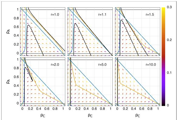
**Figure 1.** Phase portraits. Flow diagrams for different values of r. Blue, yellow and black lines correspond to  $\dot{\rho}_D=0$ ,  $\dot{\rho}_C=0$ ,  $\dot{\rho}_A=0$  nullclines, respectively. The intersections of nullclines show the fixed points. The arrows indicate the direction of the flows, and their color, their speed. Other parameters values are T=0.1, k=4, t=0.1. See the main text for further details.
