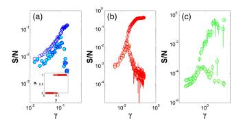
FIG. 2. Percolation of largest active cluster. Normalized size of the largest and second-largest nonaffine cluster as a function of strain for experiments (a), atomistic simulations (b), and mesoscale simulations (c). In all cases, the largest cluster grows with strain to a plateau, while the second largest cluster decays after some critical strain. The transition defines the critical strain  $\gamma_c$ . Inset in (a) shows percolation of largest cluster (P=1) versus strain in experiment.
